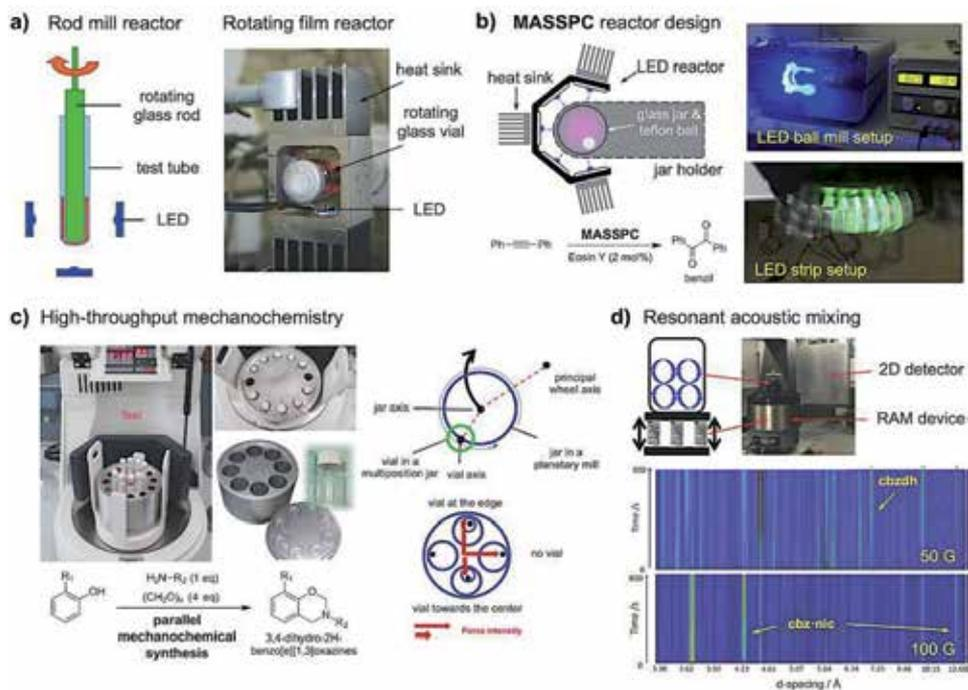
**Figure 16.** (a) Rod mill and rotating film reactors for solvent-free photocatalysis. (b) MASSPC reactor for simultaneous ball milling and LED irradiation. (c) A multiposition jar adapter for planetary ball milling and the lunar motion of vials in the adapter. (d) Resonant acoustic mixing device and the effect of acceleration on the cocrystallization of carbamazepine and nicotinamide.
