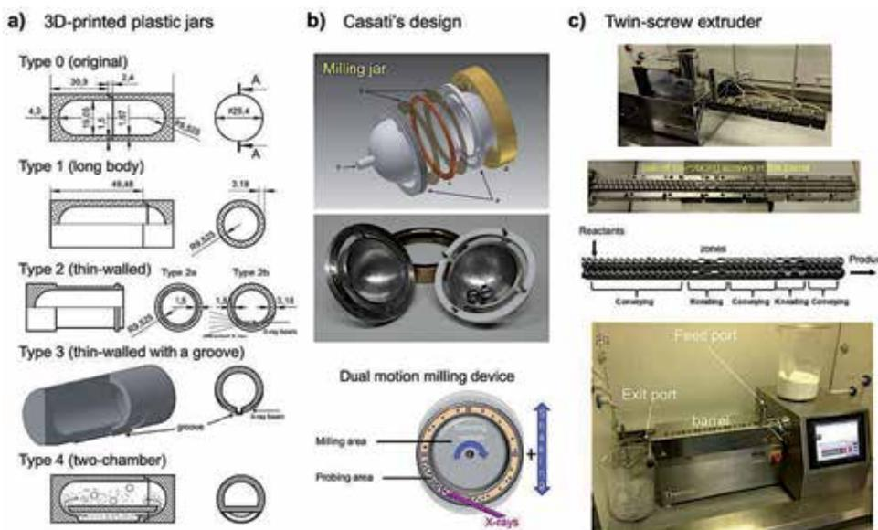
**Figure 17.** (a) Different types of 3D-printed plastic jars. (b) Casati's design of a probing jar and a dual motion ball mill. (c) Twin-screw extruder and its components.
