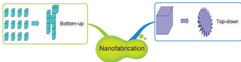
Figure 48. The two approaches to nanofabrication: the top-down and the bottom-up approaches.
