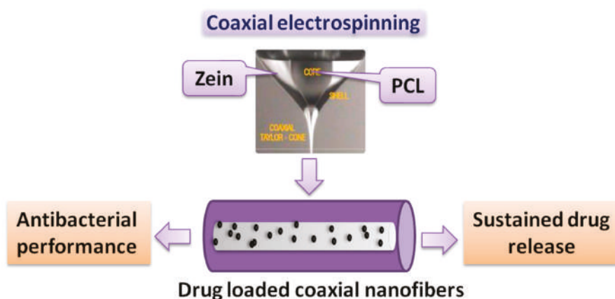
Figure 6. Structure diagram of coaxial fiber [97]. © Elsevier Inc. All rights reserved 2016.
