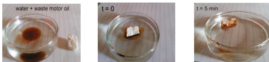
Figure 9. Waste motor oil absorption test of the silanized cellulose aerogel with MEMO silane.
