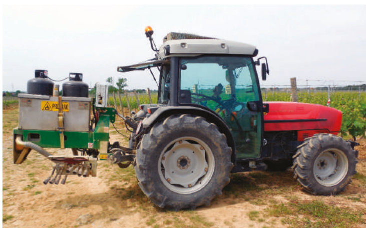
Figure 2. The flaming machine PFV-600 (Officine Mingozi, Ferrara, Italy) coupled with a SAME Frutteto 100 (SAME, Treviglio, Italy) tractor.
