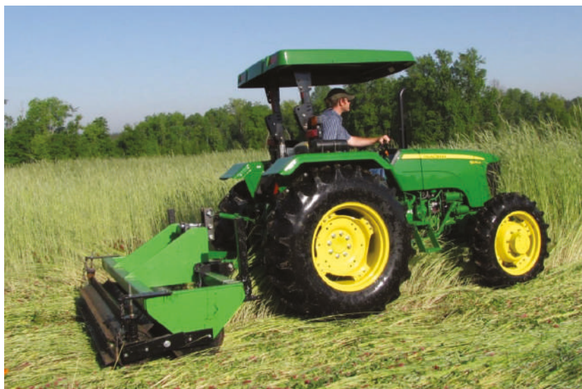
Figure 3. Side view of the experimental patented two-stage roller/crimper with two adjustable compression springs to set crimping force of the secondary crimping drum.
