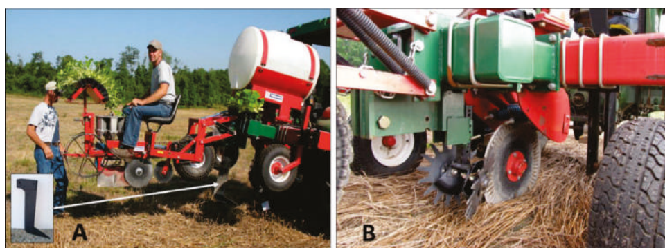
Figure 4. (A) RJ Equipment® no-till transplanter, with the additional custom designed sub-frame to accommodate a custom subsoiler shank (subsoiler used is pointed by arrow) for a single combined subsoiling and transplanting operation. (B) Row cleaners were mounted for cover crop residue management.
