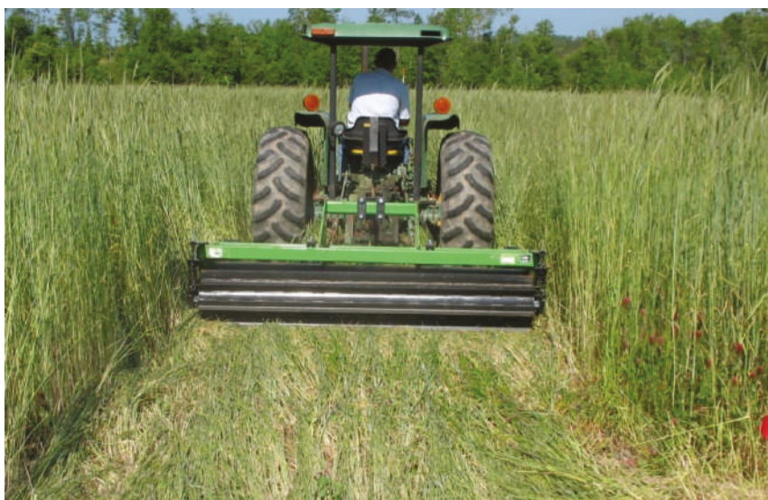
Figure 2. Cereal rye crimson clover mixture being rolled/crimped by an experimental patented 1.8 m wide 2-stage roller/crimper.
