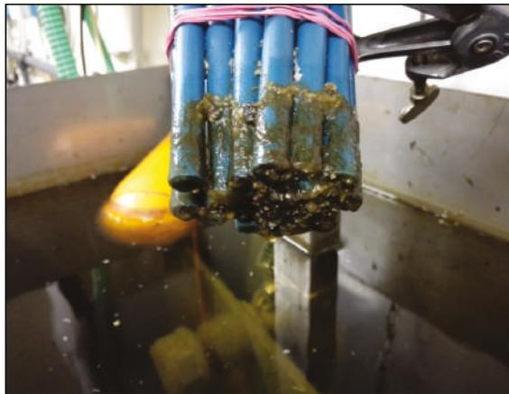
**Figure 16.** The sensor array after long-term online measurements at an aeration water plant. The sensors were cleaned by intensive washing. In spite of significant contamination, the sensors were stable for at least two months [79].
