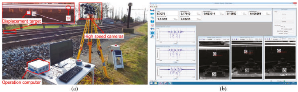
Figure 6. Wayside monitoring. (a) System setup. (b) The screen of displacement measurements.
