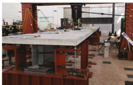
Figure 3. Verified by fatigue tests on bridge model.
