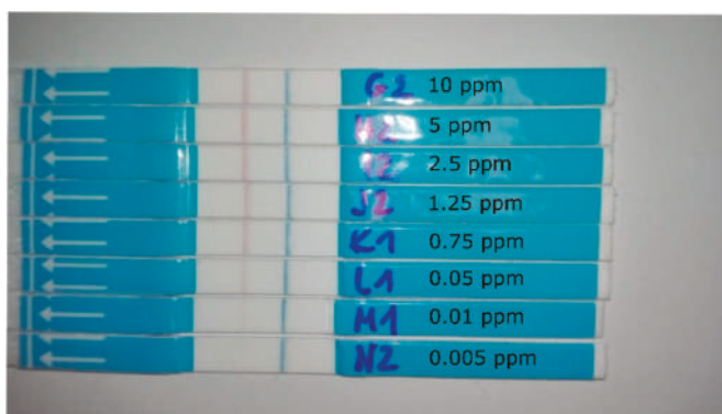
Figure 5. A set of LFAs used to build a calibration curve for gluten quantification with various smartphones. The concentrations of gluten used are indicated.
