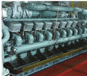
**Figure 12.** The diesel engine with 20 cylinders.
