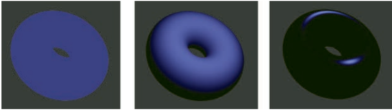
FIGURE 6.3 Ambient, diffuse, and specular lighting on a torus-shaped surface.
