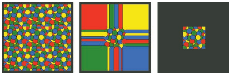
FIGURE 5.4 Texture wrap settings: repeat, clamp to edge, clamp to border.
