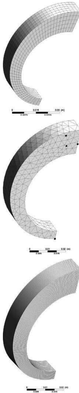
Figure 5. Division of geometrical model of the heat flux tube into finite elements; (a) hexahedral mesh—1150 elements hex8, 1692 nodes; (b) tetrahedral mesh—1909 elements tet4, 518 nodes; (c) hexahedral mesh—59520 elements hex8, 66759 nodes.
