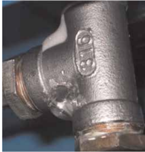
Figure 22. Source of leakage identified after on-site inspection.
