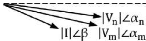
Figure 5. Phasor diagram for upstream and downstream node voltage and line current for Case 1.
