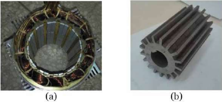
Figure 28. 12-slot/17-pole FRPMM prototype: (a) stator; (b) rotor.
