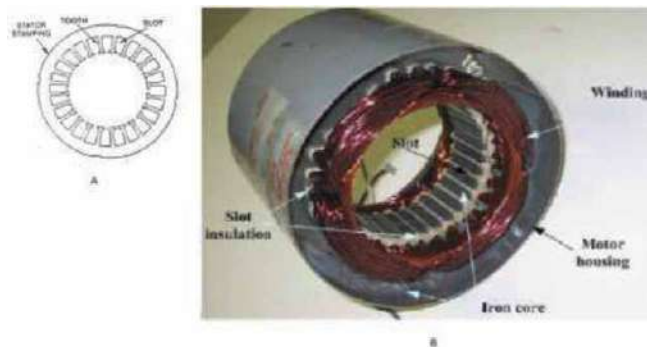
Figure 1. (A) Stator stamping with slots of induction motor. (B) Stator of Induction Motor.
