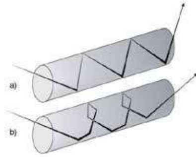
Figure 13. Rays taking meridional (a) and helical (b) forms in an optical fiber [12].
