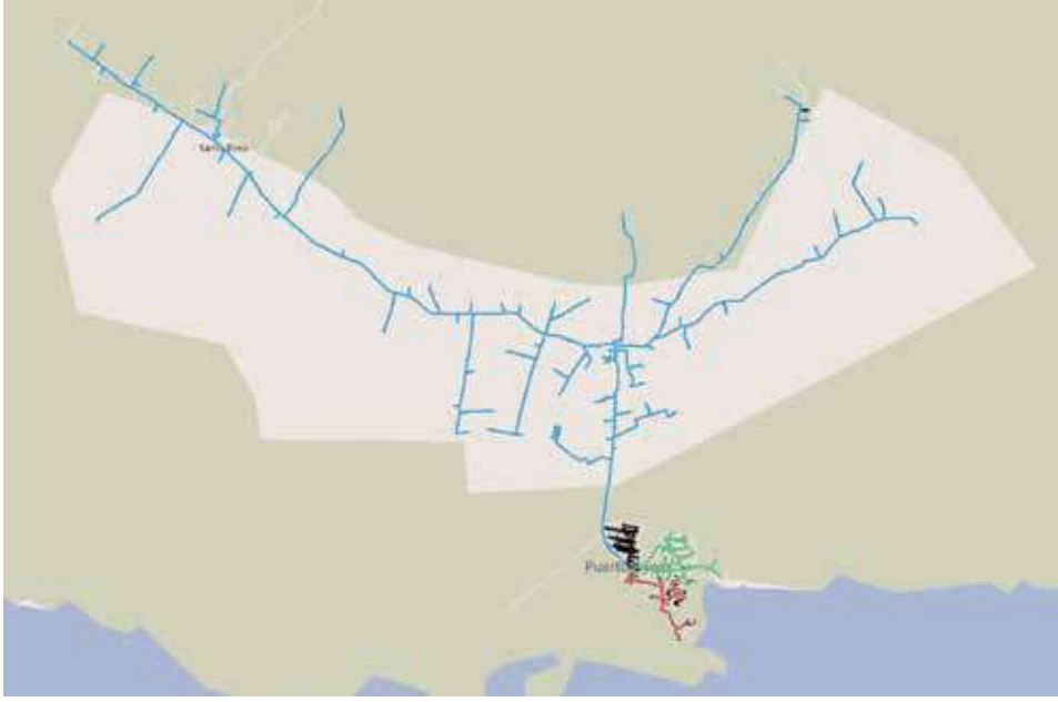
Figure 3. Medium voltage distribution system in Santa Cruz [30].
