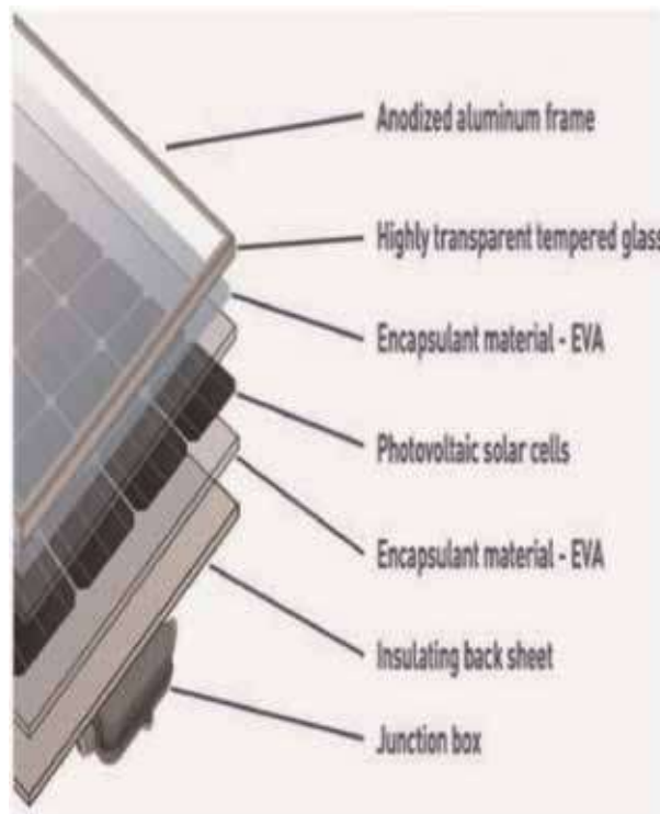
Figure 1. The structure of a PV module.
