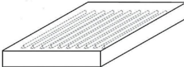
**Figure 1.** Micro-heat pipe array in silicon wafer.
