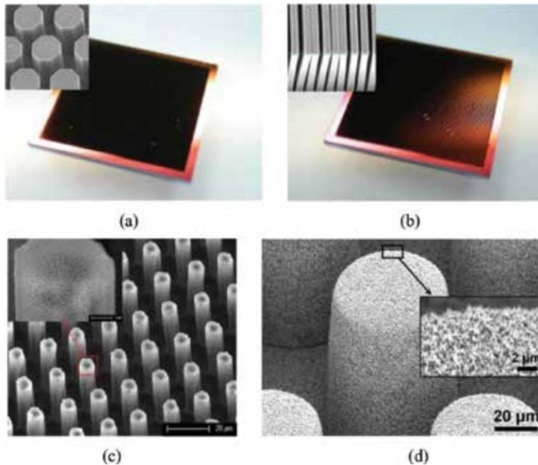
**Figure 14.** SEM images of micro-/nano-hierarchical wicking structures for micro-vapor chamber: (a) biwick structure composed of cylindrical CNT pillars [81]; (b) biwick structure composed of straight CNT stripes [81]; (c) Ti pillar array with oxidized hairlike NST(nanostructured titania) [82]; (d) nanostructured Cu micro-posts [83].
