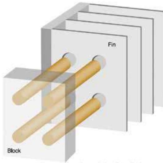
Figure 17. Block-to-fin applications.
