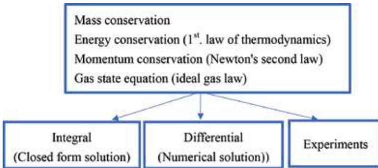
Figure 5. Three methods for solving heat-dissipated problems.
