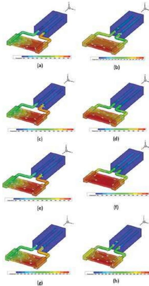
**Figure 8.** Temperature profile on the evaporator surface,  $T = 30$  s for heat fluxes (a), (b)  $11594.2 \text{ W/m}^2$  (c), (d)  $13043.48 \text{ W/m}^2$ , (e),(f)  $14492.75 \text{ W/m}^2$ , and (g),(h)  $15971.01 \text{ W/m}^2$ .
