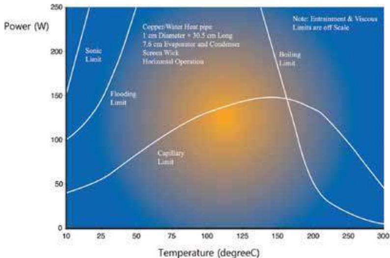
**Figure 7.** Performance limitations with respect to the temperature.
