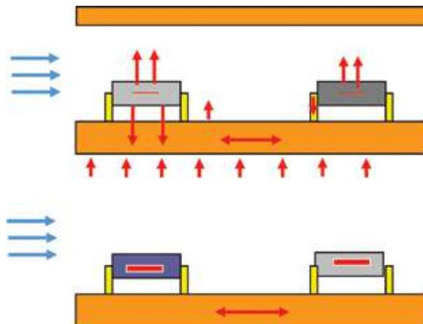
Figure 3. Heat transfer mechanism between each PCB.
