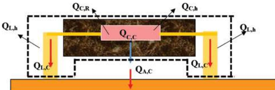
Figure 6. Heat transfer diagram outside the chip.
