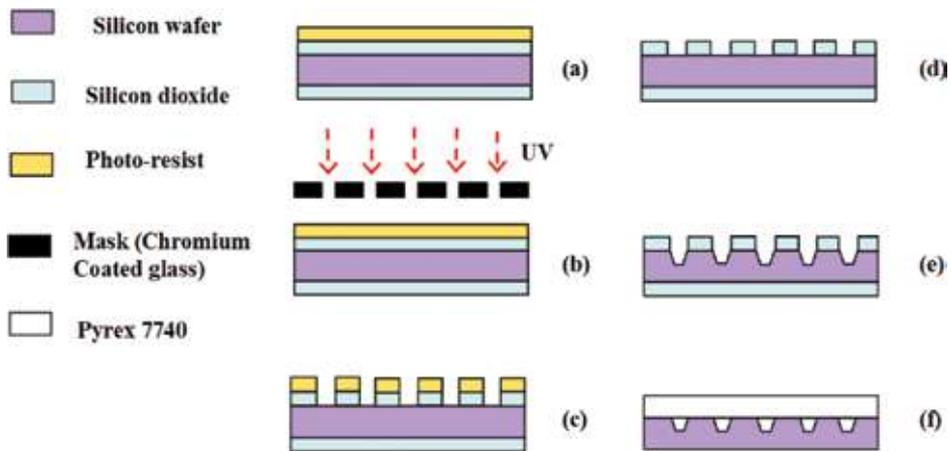
**Figure 4.** Fabrication processes of a MEMS-based MHP: (a) spin coating photoresist, (b) UV exposure, (c) BOE etching (d) wet etching, (e) HF etching silicon layer, and (f) silicon-to-glass anodic bonding.
