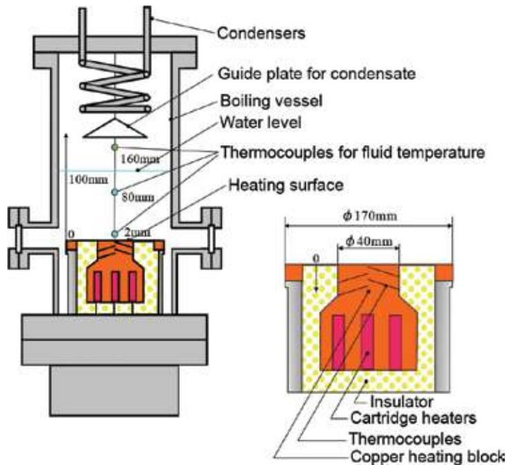
Figure 5. Outline of pool boiling experimental apparatus.
