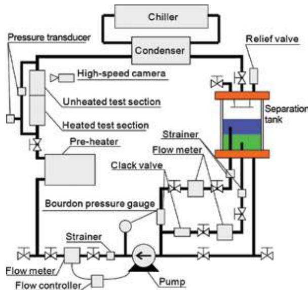
Figure 12. Test loop [21].
