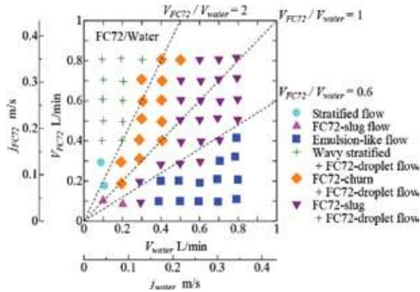
Figure 14. Flow pattern map for FC72/water. [21]
