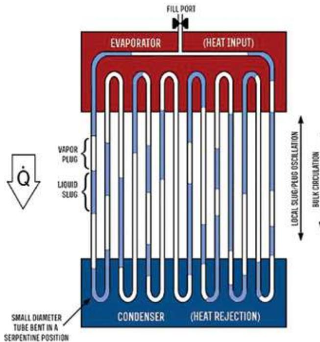
**Figure 8.** Schematic of an oscillating heat pipe [33].
