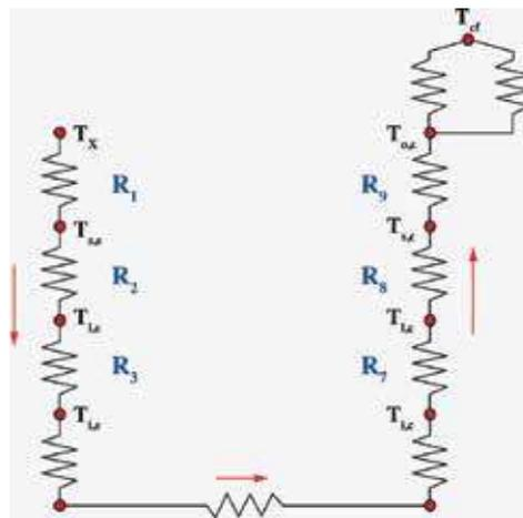
**Figure 13.** Thermal resistance network.
