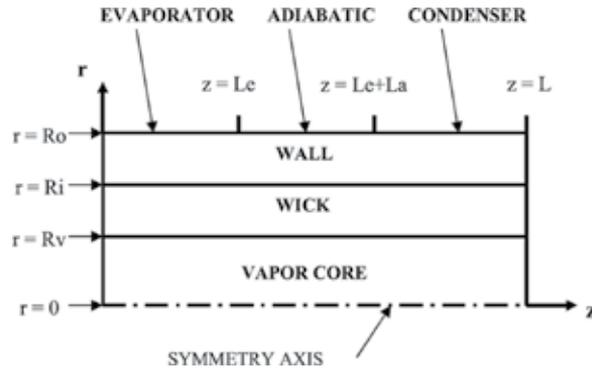
Figure 9. Coordinate system of the heat pipe [38].
