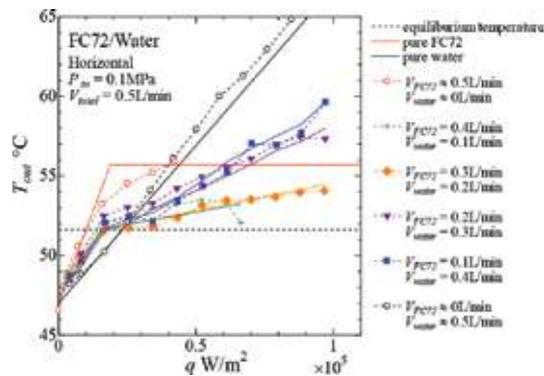
Figure 15. Outlet fluid temperature versus heat flux.
