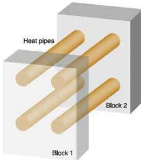
Figure 18. Block-to-block applications.
