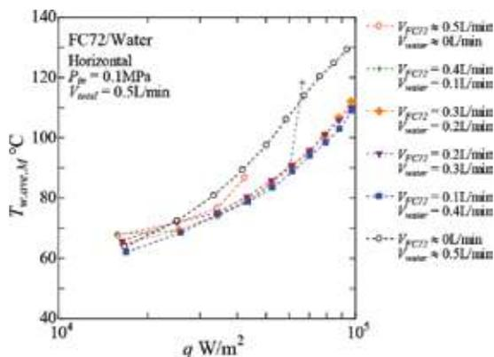
**Figure 17.** Wall temperature versus heat flux at midstream.
