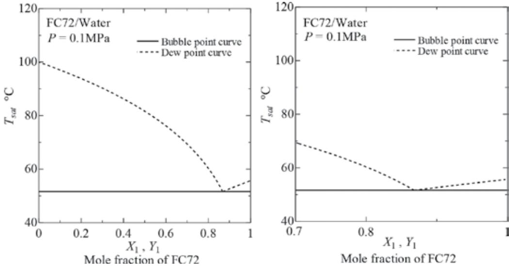
Figure 3. Phase equilibrium diagram of FC72/water mixture.
