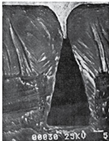
**Figure 5.** A vapor-deposited micro-grooved heat pipe [17].
