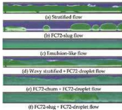
Figure 13. Typical flow patterns of FC72/water [21].
