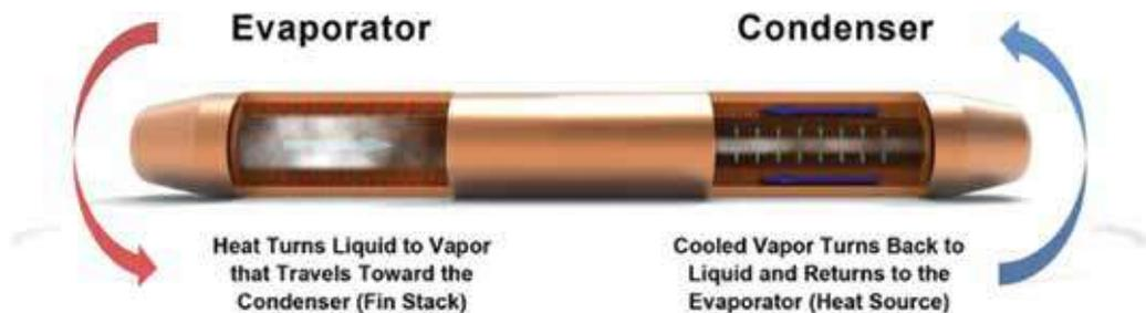
**Figure 5.** Cylindrical heat pipe [24].
