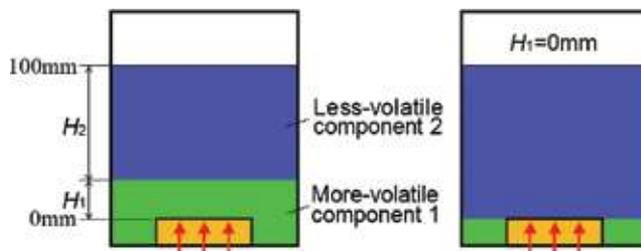
Figure 6. Condition representing volume ratio of immiscible liquids [9].
