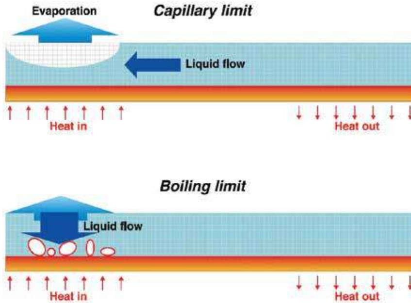
Figure 8. Capillary limit and boiling limit.
