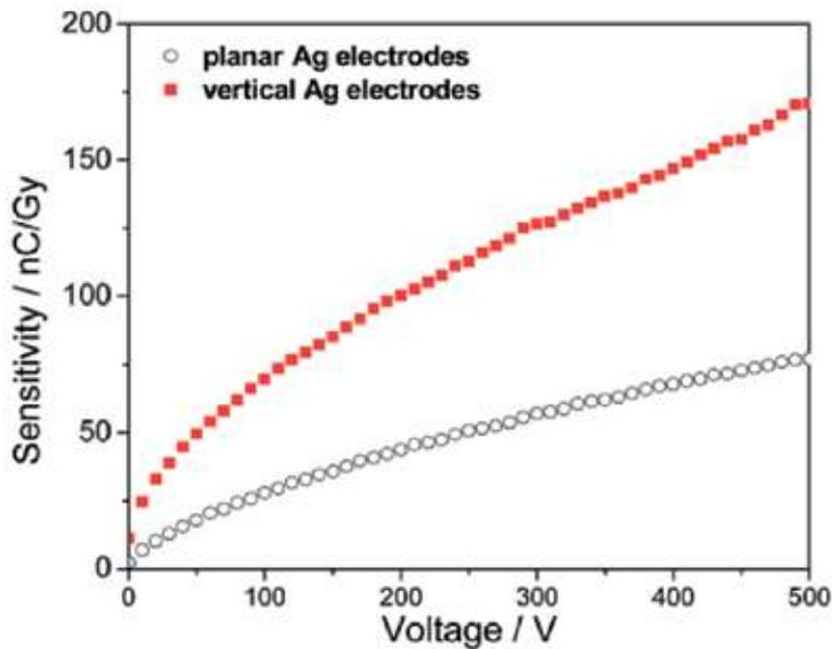
**Figure 6.** Comparison between the sensitivity values at different bias voltages for a 4HCB-based detector under 35 keV X-ray irradiation in the planar (black circles) and vertical (red squares) electrode configuration [26].
