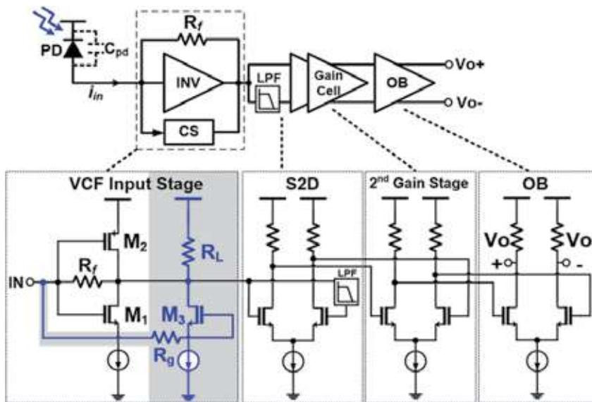
**Figure 9.** Schematic diagram of the VCF-TIA.
