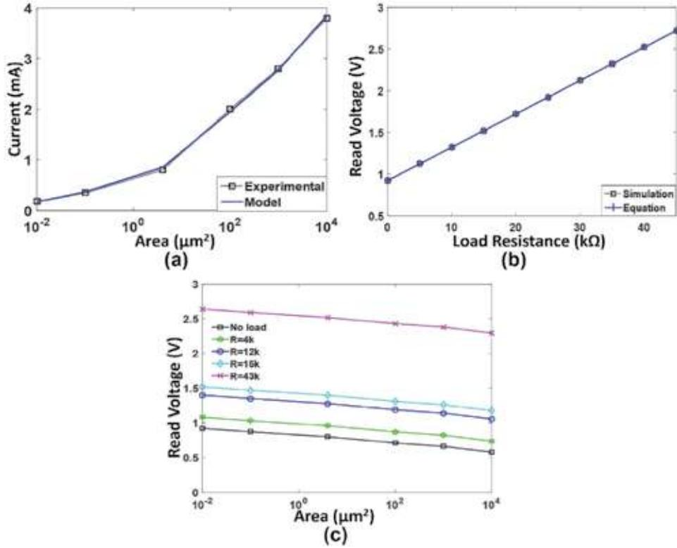
**Figure 6.** (a) The diode current versus diode area @ bias voltage = 1 V and no-load resistance. The data are from the implemented diode Verilog-A model verified against experimental data in [23]. (b) The required read voltage to supply  $I_{Read} = 40 \mu A$  with diode area scaling for various  $R_{load}$ . (c) The required read voltage for the diode to supply  $I_{Read} = 40 \mu A$  versus different  $R_{load}$  using both Verilog-A model simulation and Eq. (1) [18].
