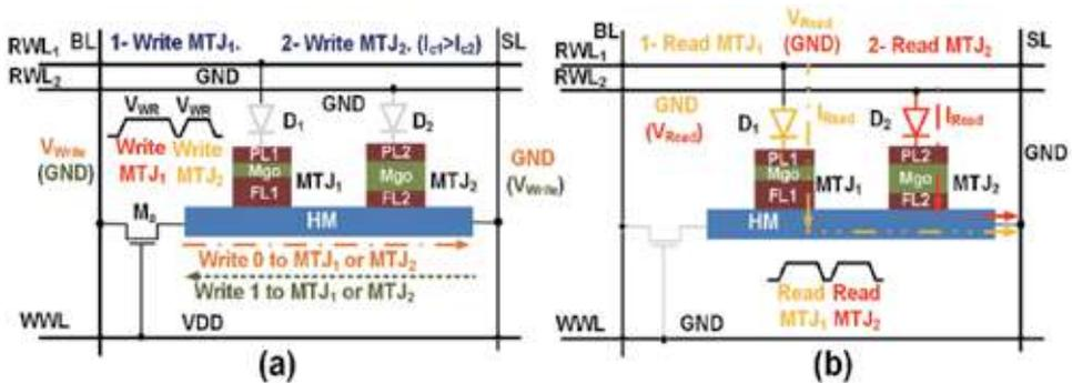
**Figure 5.** Proposed MBC-DD SOT-MRAM cell in the (a) write and (b) read operations [18].
