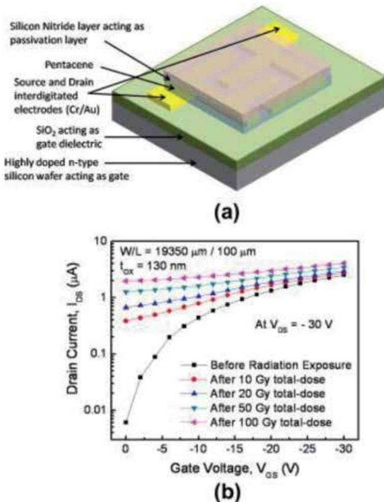
**Figure 3.** (a) Schematic of a pentacene OFET in bottom gate bottom contact configuration with interdigitated source and drain electrodes using a silicon nitride passivation layer, and (b)  $I_d$ - $V_g$  characteristics for a Pentacene OFET with exposure to increasing dose of ionizing radiation [18].
