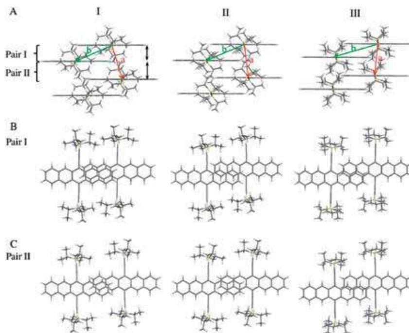
**Figure 3.** Comparison of the three major polymorphs of TIPS-pentacene in their  $\pi$ - $\pi$  stacking (A) and molecular offset along the conjugated backbone (B, C) as obtained from the crystallographic refinement calculations [15]. Copyright 2014, American Chemical Society.
