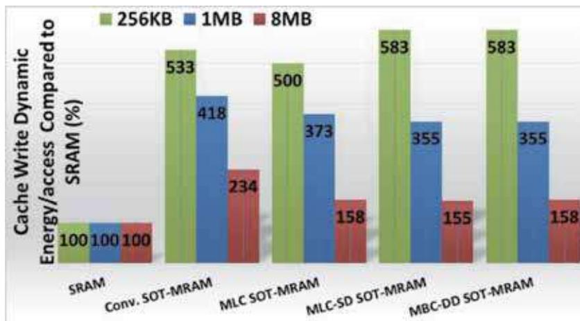
**Figure 12.** Cache write dynamic energy per access comparison of the SRAM, conventional, P-MLC, MLC-SD, and MBC-DD SOT-MRAMs for different capacity relative to SRAM assuming improved high-speed SOT-MT technology (e.g. type-x reported in [13]).
