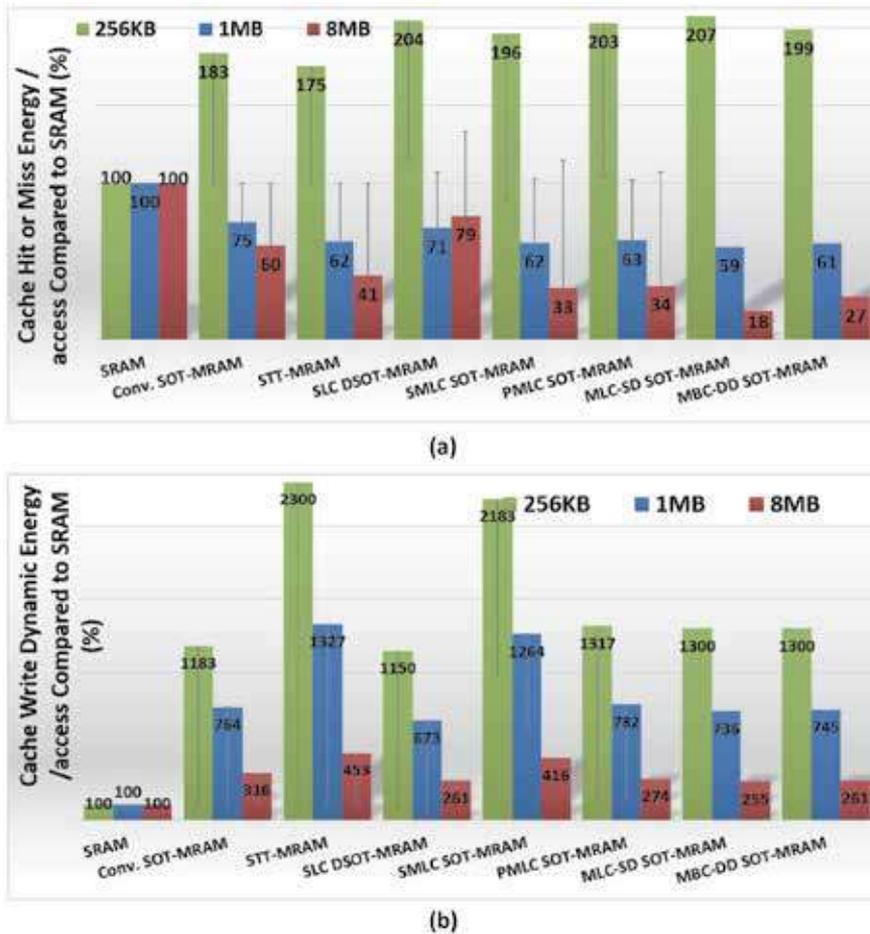
**Figure 11.** Comparison of the SRAM, STT-MRAM, conventional, SLC diode-based, S-MLC, P-MLC, MLC-SD, and MBC-DD SOT-MRAMs for different capacities relative to SRAM from (a) cache hit/miss energy per access perspective and (b) cache write dynamic energy per access perspective.
