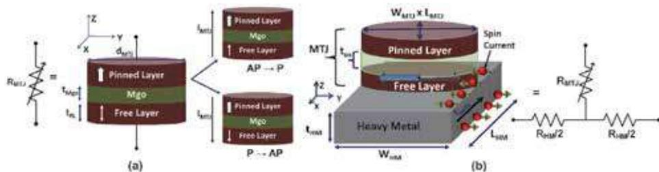
**Figure 1.** (a) Two-terminal MTJ with two magnetization configurations reflects two resistance states depending on the write current direction if STT technology is used. (b) Three terminal SOT-MTJ.
