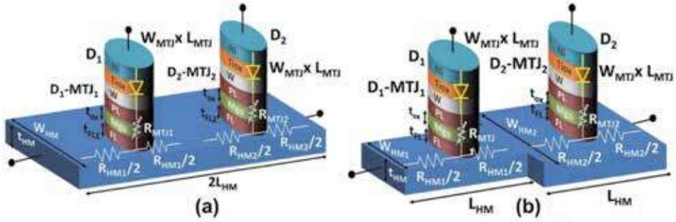
**Figure 4.** 3D structure of the proposed dedicated diode multi-bit per cell (MBC) DD SOT-MRAM with (a) uniform HM electrode and MTJs with different  $\tau_t$  [18], (b) different HM width and MTJs with similar  $\tau_t$  [18].
