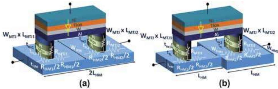
**Figure 7.** 3D structure of the proposed shared diode multi-level cell (MLC) SOT-MRAM with (a) uniform HM electrode and MTJs with different  $\tau_t$  [17], (b) different HM width and MTJs with similar  $\tau_t$  [17].
