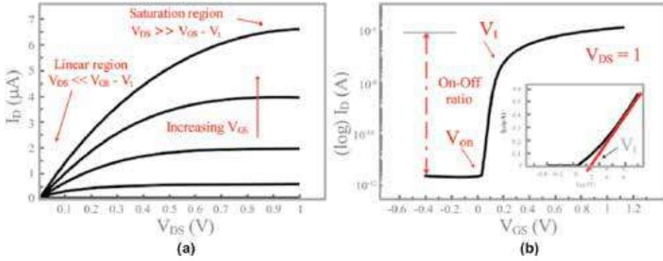
**Figure 3.** Typical output (a) and transfer (b) characteristics of a low voltage OFET operating at 1 V.
