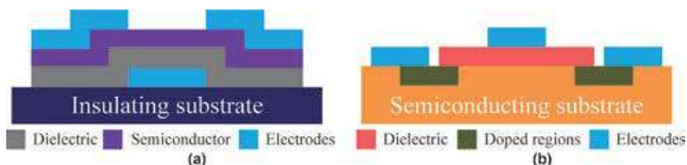
**Figure 1.** Typical structures of (a) a bottom-gate top-contact TFT and (b) a MOSFET. Doped regions refer to the MOSFET source and drain regions.
