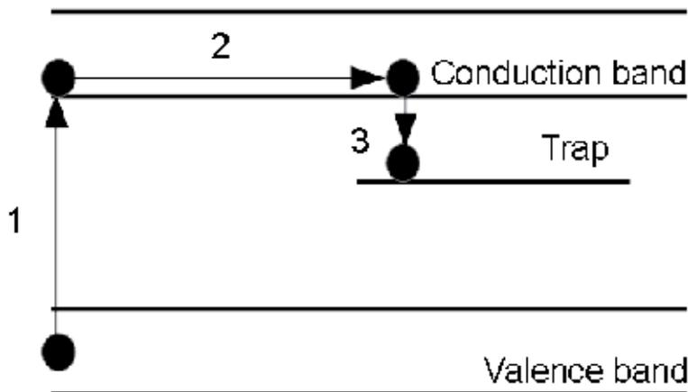
**Figure 1.** Optically stimulated luminescence for dosimetry: An electron (1) is excited by a light source into the conduction band, (2) migrates through it and (3) falls into a trap emitting a characteristic light proportional to the number of traps previously induced by ionizing radiation.
