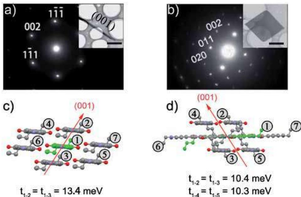
**Figure 8.** SAED and TEM images of (a) the  $\alpha$ -phase and (b) the  $\beta$ -phase crystals (the scale bar is  $5\ \mu\text{m}$ ). The transfer integrals of (c) the  $\alpha$ -phase and (d) the  $\beta$ -phase crystals along the  $(001)$  directions. The molecules in panels e and f are colored differently only for clarity purposes [55]. Copyright 2018, American Chemical Society.
