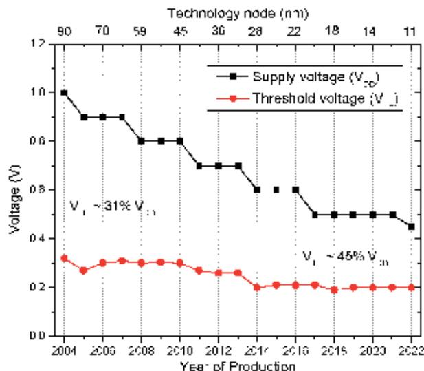
**Figure 1.** Scaling the supply voltage and threshold voltage in time.
