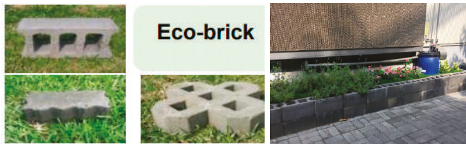
Figure 8. Eco-brick made from waste cinder and used in the factory.
