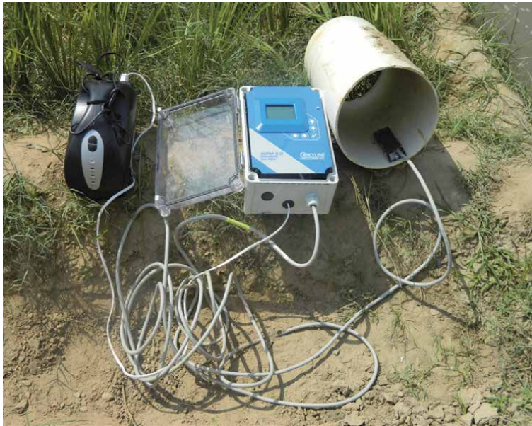
Figure 8. Area Velocity Flow Meter for calculating the irrigation water applied.
