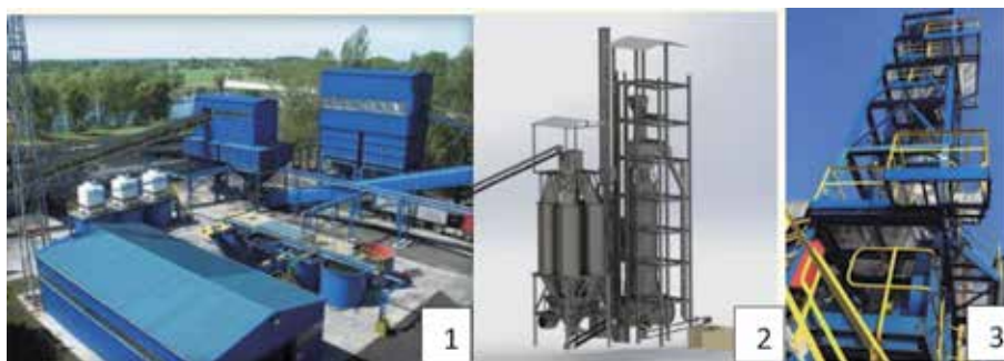
Figure 6. Representative continuous BC production systems: (1) Polchar production facility, GCS's (2) vertical retort process and (3) vertical retort.
