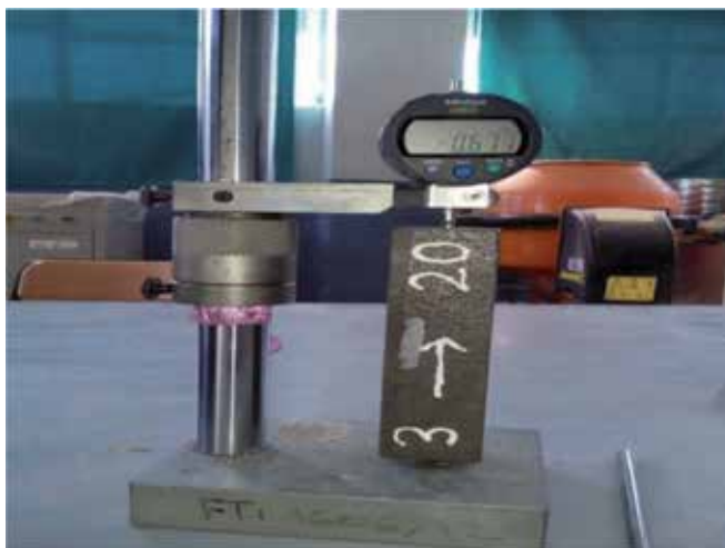
Figure 14. Shrinkage measurement on prismatic test piece.
