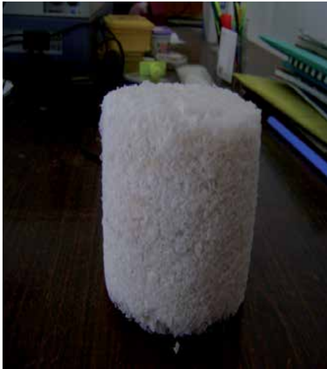
Figure 13. Shredded PTFE scrap after pre-heating treatment
