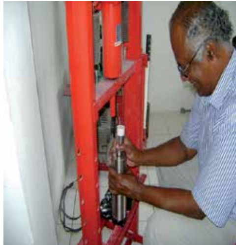
Figure 17. Mixture being cold pressed into pellet.
