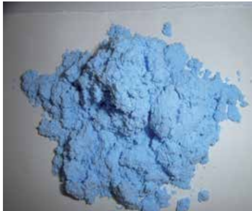
Figure 4. A blue pigment (3%) mixed non free flow PTFE powder.
