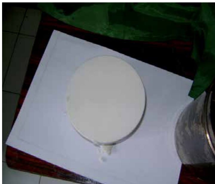
Figure 14. Pre-sintered scrap powder
