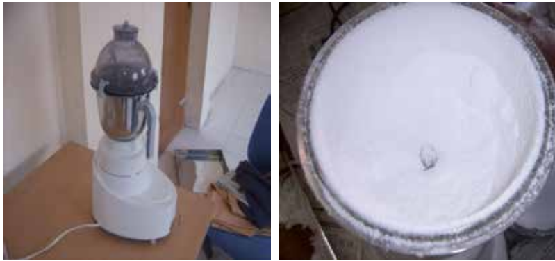
Figure 16. Ground PTFE powder being mixed with virgin PTFE powder.
