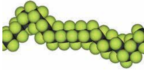
Figure 1. Typical intertwined PTFE polymer. Due to strong intermolecular forces, the polymer chains are tangled. Due to its chemical inertness, PTFE cannot be cross-linked.
