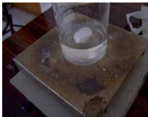
Figure 3. PTFE is hydrophobic – water repellant
