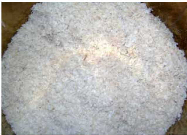
Figure 11. Charred organic impurities on pre-heating the shredded scrap
