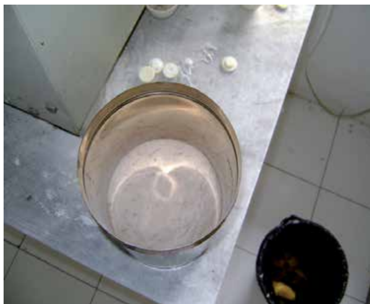
Figure 15. Ground scrap powder after pre-sintering
