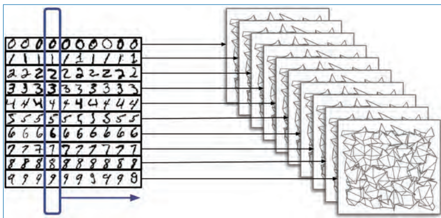
Figure 7.28. Network architecture used for training. A source layer displays a series of examples of handwritten digits; each example from a particular class is projected to the target layer corresponding to that class.
