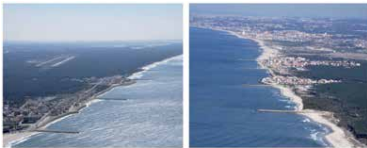
Figure 3. Urban seafronts protected by sea walls and groins. These residential areas are located at the western Portuguese coast (Mira on left and Esmoriz-Cortegaça on right) and are only maintained at the expense of hard engineering projects (Courtesy of Lopes [5]).
