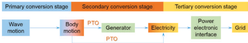
Figure 4. Main stages of wave energy conversion.
