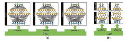
Fig. 6.2 (a) Data parallelism and (b) model parallelism
