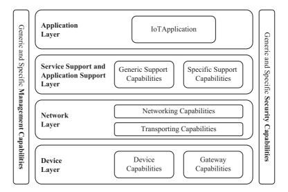
Fig. 8.1 IoT architecture. (Adapted from ITU 2012)
