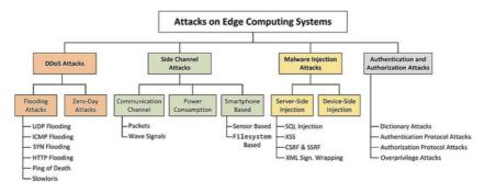
Fig. 6.1 Different types of attacks against edge computing systems (Xiao et al. 2019)
