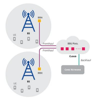
Fig. 3.2 A general architecture of a C-RAN cellular network
