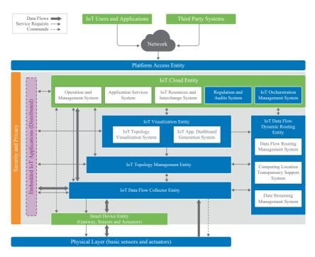
Fig. 1.9 The SAT-IoT Architecture. (Adapted from Peña and Fernández 2019)
