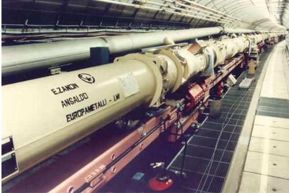
**Fig. 6.30** View of the two independent storage rings for electron and proton acceleration in HERA. The super conducting proton lattice is placed on top of the conventional electron ring
