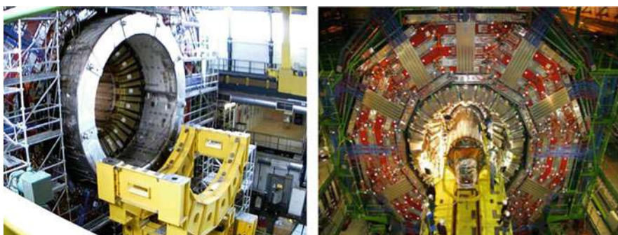
Fig. 16.4 Left: picture of the CMS superconducting solenoid, as integrated with the barrel muon system (outside) and with the barrel hadron calorimetry (inside). Right: picture of the insertion of the CMS silicon-strip tracker into the barrel crystal calorimeter
