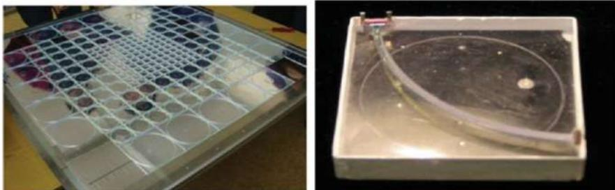
**Fig. 22.16** Picture of a prototype readout plane for a highly segmented tile calorimeter (left) and one scintillator tile with wavelength shifting fibre and SiPM readout (right) [70]
