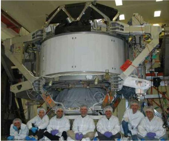
**Fig. 18.16** The AMS-02 spectrometer during its integration at CERN in 2009 in the final flight configuration with the permanent magnet
