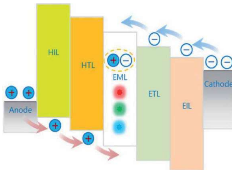
Figure 1. Structure of an OLED device.
