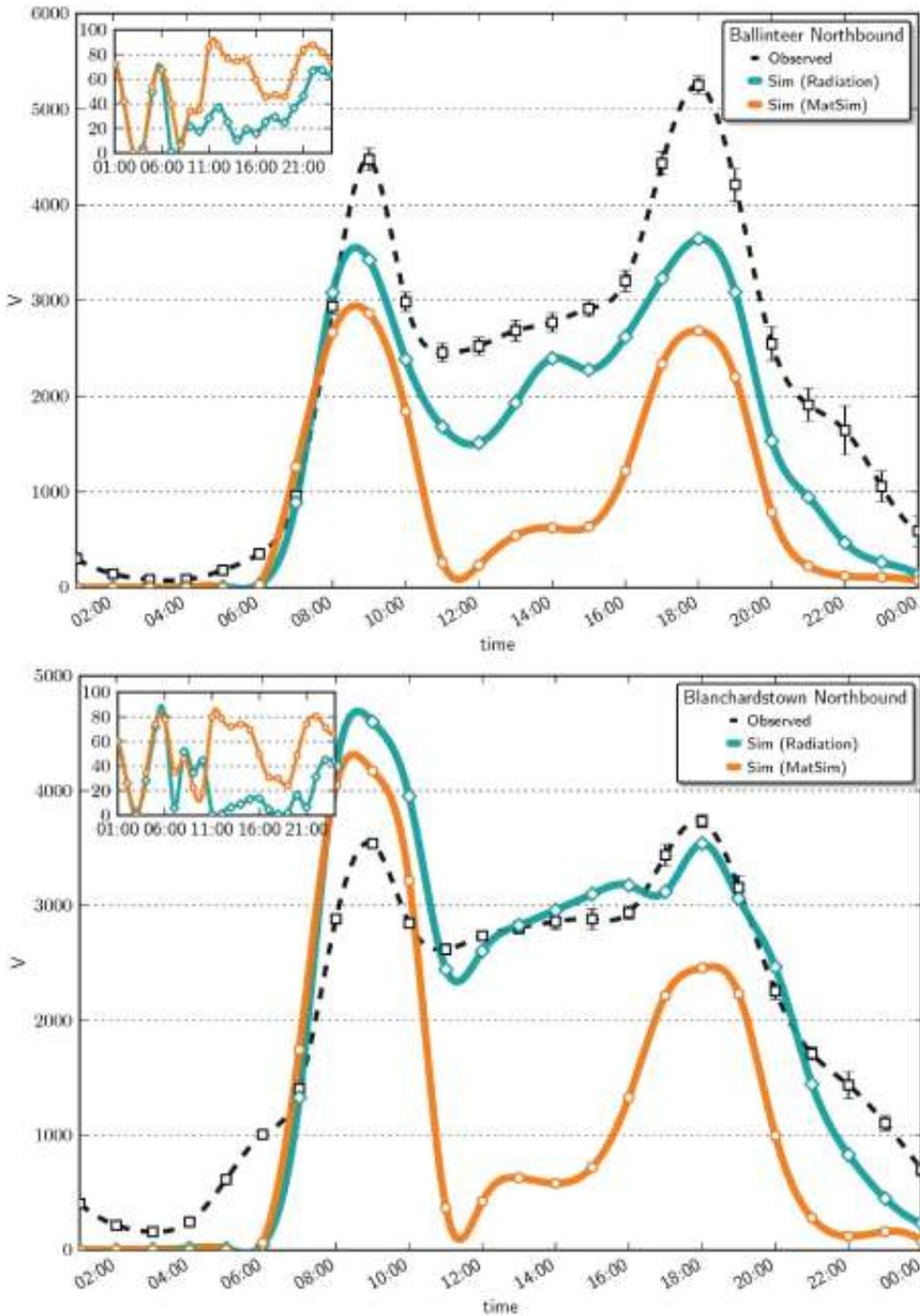
**Figure 67.2:** Hourly observed traffic volumes (dashed line) compared to the estimated traffic volumes produced by MATSim using the radiation model (green line) and nearest neighbor model (orange line).
