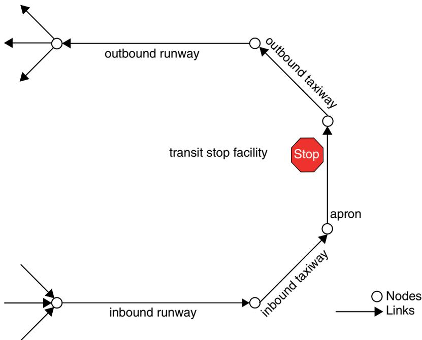
**Figure 68.1:** Layout of airports in the air transport network: In- and outbound runways are modeled by separate links connected by taxiways and a link representing the apron. There the transit stop facility is attached.
