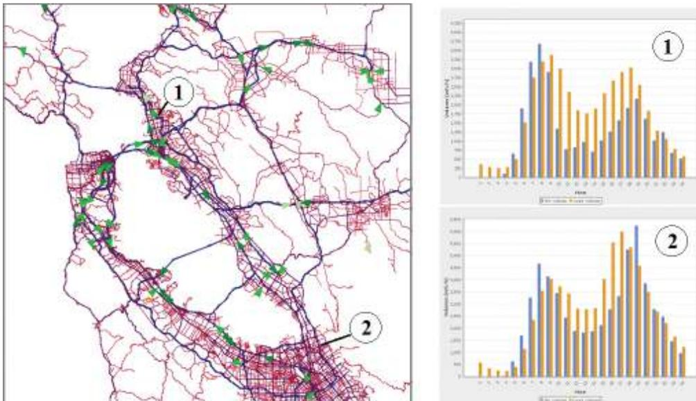
**Figure 83.2:** A sample of the simulated vehicles and the examples of the observed (light/orange) and simulated (dark/blue) counts at two particular validation locations. Secondary trips, mainly occurring at midday, were not included in this scenario.
