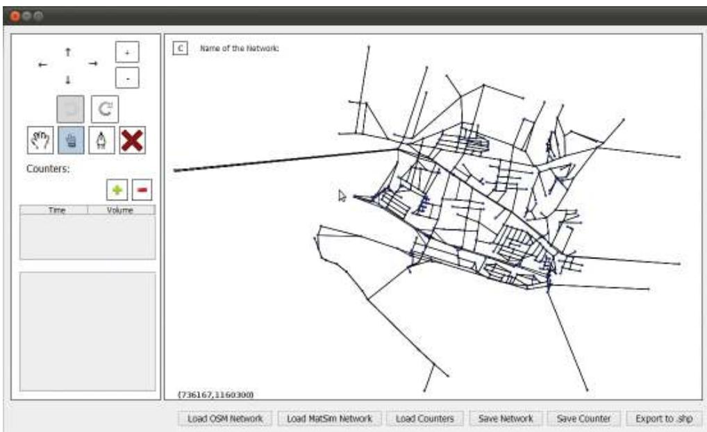
**Figure 65.2:** Interface of the software tool developed in Java showing the area studied. Blue dots over the roads in the map represent the counters positioned in the area to capture vehicle flow used as input for the simulation.
