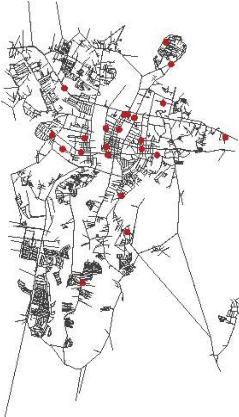
**Figure 78.2:** Spatial coverage of road network and locations of facilities in the network: it has 73.2 square kilometers including land and surrounding river and coastal areas. The facilities are mapped based on its actual geographical x and y coordinates in the road network. There are 23 facilities located in its nearest link in the network. These are: 10 hospitals, three fire stations, eight police stations and two evacuation centers.
