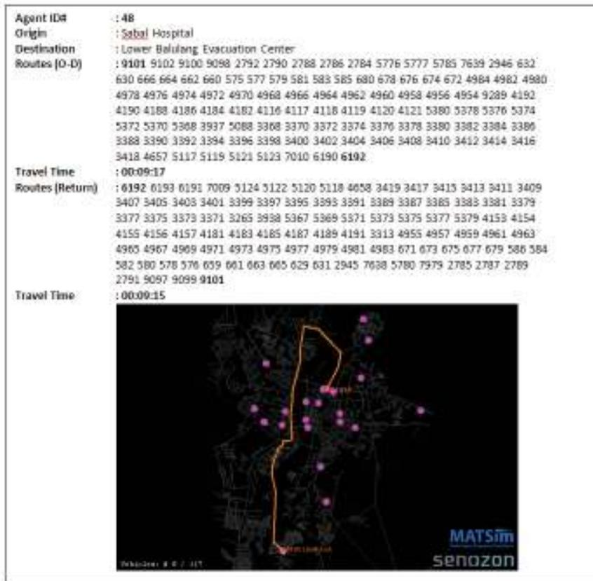
**Figure 78.5:** Screenshot of SCENARIO 2 (with bridge closures) using agent ID#48. DRVs trip starting from the Sabal Hospital (Origin) passing Kauswagan-Puntod Bridge going to Balulang Evacuation Center dropping point (destination) then back to its origin.
