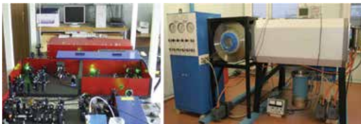
Figure 4. THL-30: Photographs of the Ti:sapphire front end (left) and XeF(C-A) amplifier (right).
