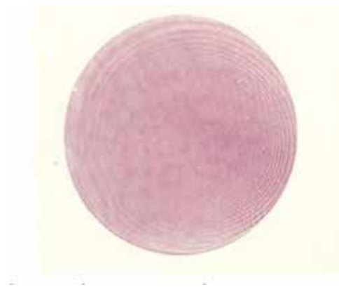
Figure 12. Imprint of the output laser beam with 2.5 J energy.
