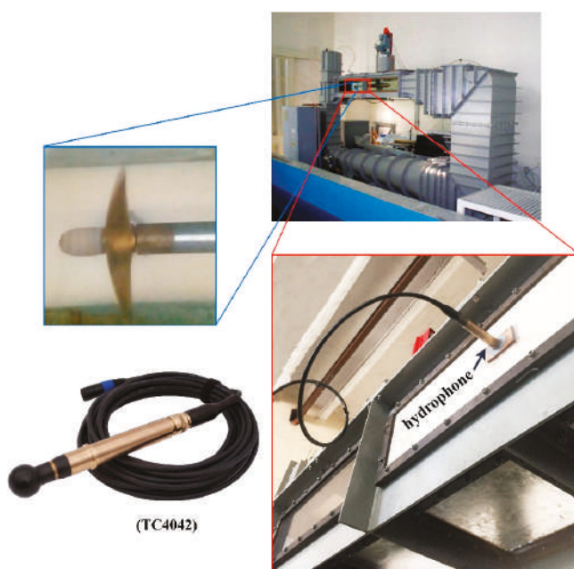
Figure 10. Arrangement of TC4042 hydrophone on cavitation tunnel.
