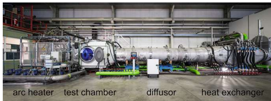
Fig. 6 Arc-heated wind tunnel L3K at DLR, Cologne
