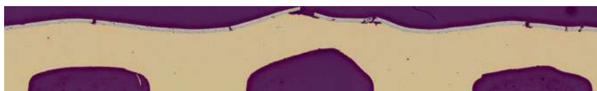
Fig. 6 Cross section through the central cooling channels: Large deformation of the thin copper wall caused partial coating delamination
