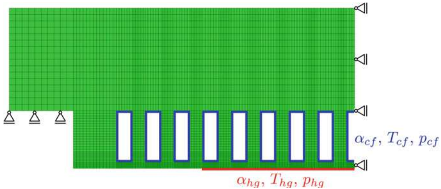
Fig. 5 FE model of the fatigue specimen with thermal and mechanical boundary conditions
