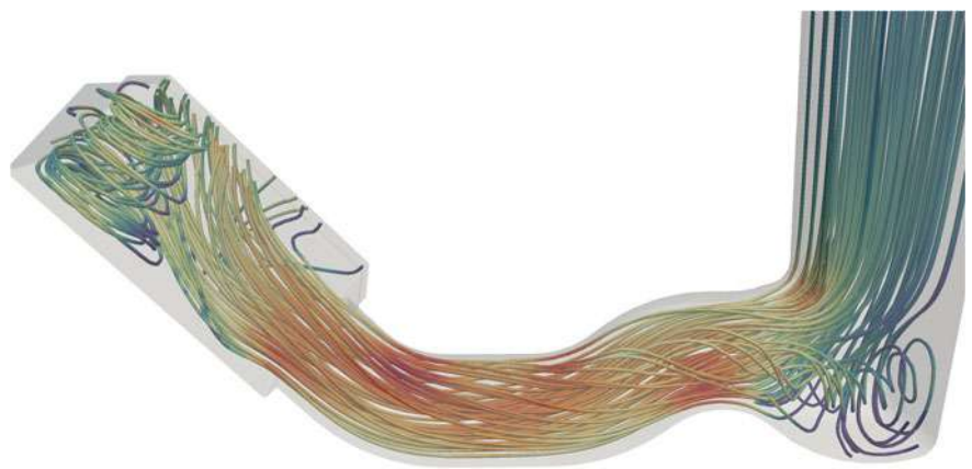
Fig. 4.14 Simulated static flow conditions in the lower area of the mold at the end of the casting process
