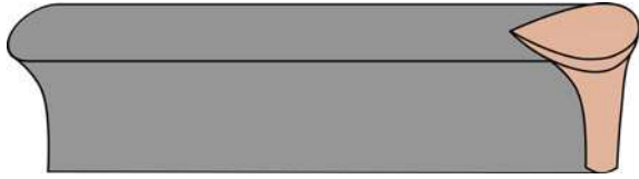
Fig. 18.20 3D-view of fusion zone (dark grey) and molten weld pool (red)
