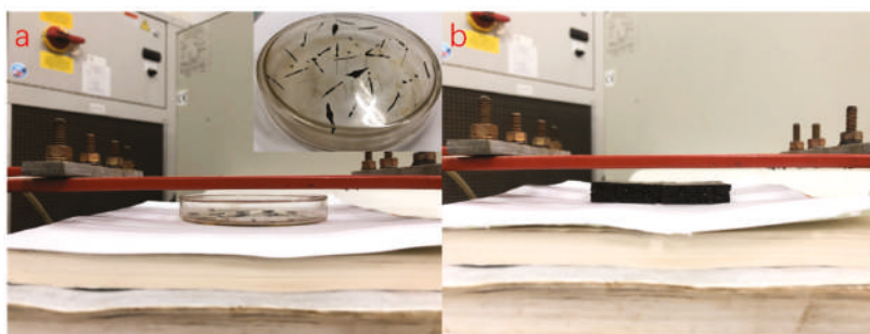
Figure 5. Induction heating test of Dramix asphalt-fibers (a) and asphalt concrete (b).
