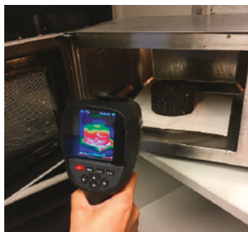
Figure 2. Surface temperature measurement of the specimen in the microwave oven.
