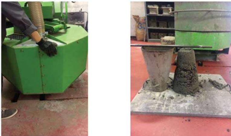
**Figure 5.** Concrete mixer (left); concrete slump test (right).
