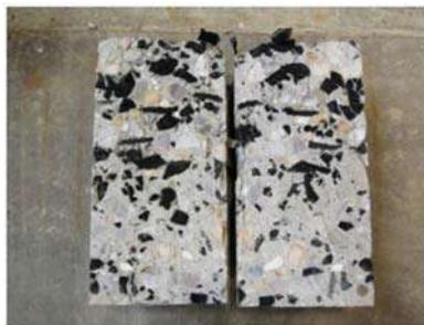
Figure 3. Crumb rubber concrete.
