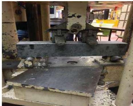
Figure 10. 4-point bending test.
