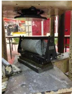
Figure 9. Splitting tensile test.
