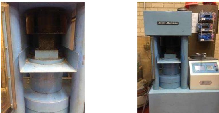
Figure 7. Compressive test setup.
