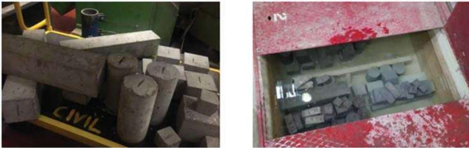
Figure 6. Specimen shapes (left); curing tank (right).
