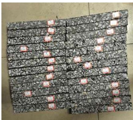
Figure 5. Standard trabecular test pieces.
