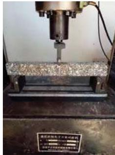
Figure 3. Fatigue test.
