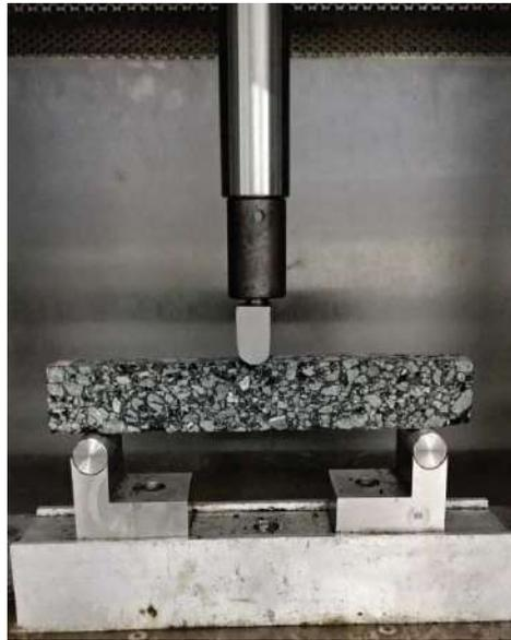
Figure 2. Three-points bending test set-up.
