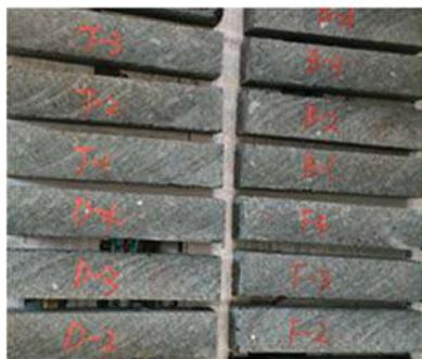
Figure 7. Samples of Four-point Bending Fatigue test.
