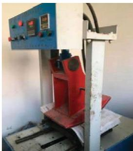
**Figure 1.** Rut board forming machine.
