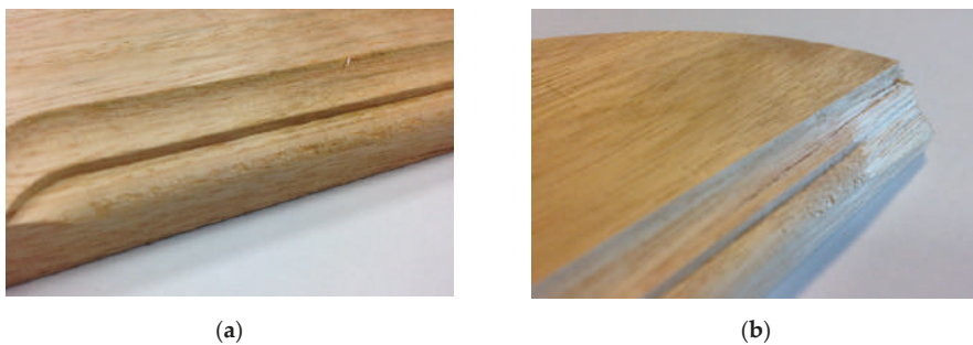
Figure 8. Examples of E. globulus with a grade of G2 (good) for fuzzy shaping side grain (a) and E. nitens with a grade of G5 (very poor) for chipped shaping side grain (b).
