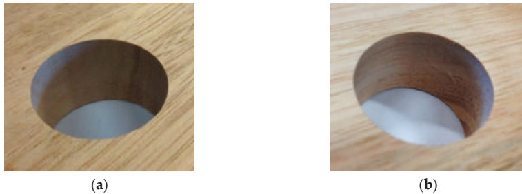
Figure 9. Examples of E. nitens with a grade of G0 (excellent) (a) and E. globulus with a grade of G2 (good) (b) for boring tear-out.
