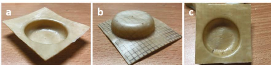
**Figure 8.** PHB/T\_RH/HMDI thermoformed tray: (a) bottom-side view, (b) top-side view and (c) bottom view.
