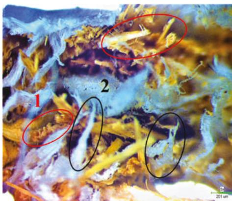
**Figure 7.** Optical micrograph of fracture surface of the hot pressed straw/LLDPE composite.
