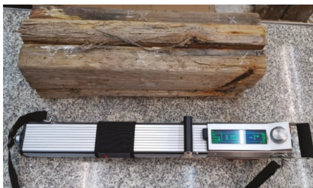
Figure 3. IML RESI PD-400S device used in tests.
