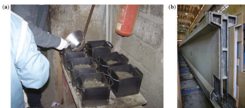
Figure 4. (a) making of the specimens; (b) manufacture of the V03 girders.
