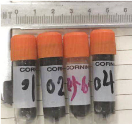
Figure 1. Paste and mortar samples encased in epoxy resin after mercury intrusion.
