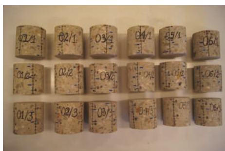
Figure 7. Core samples with height/diameter ratio h/d = 1 , obtained from samples 01–06.
