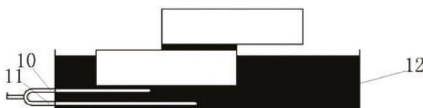
Figure 6. Test shear sample placed in the water bath.
