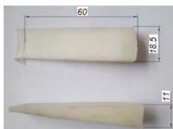
Figure 4. Geometry of the inserts with appropriate dimensions labeled.
