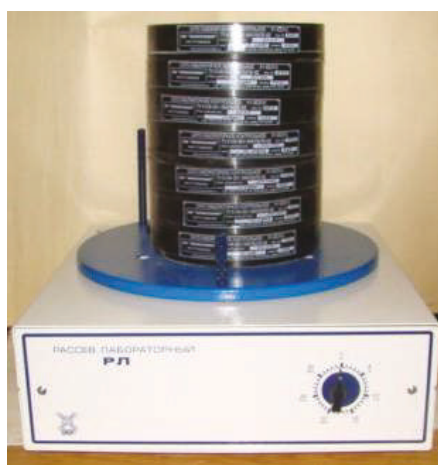
Figure 11. Laboratory planisifter RL brand with a set of sieves for determining the granulometric composition of the forage.
