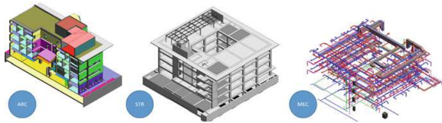
Fig. 6 As-built models of ambulatory care centre “Navile”, organised per disciplines
