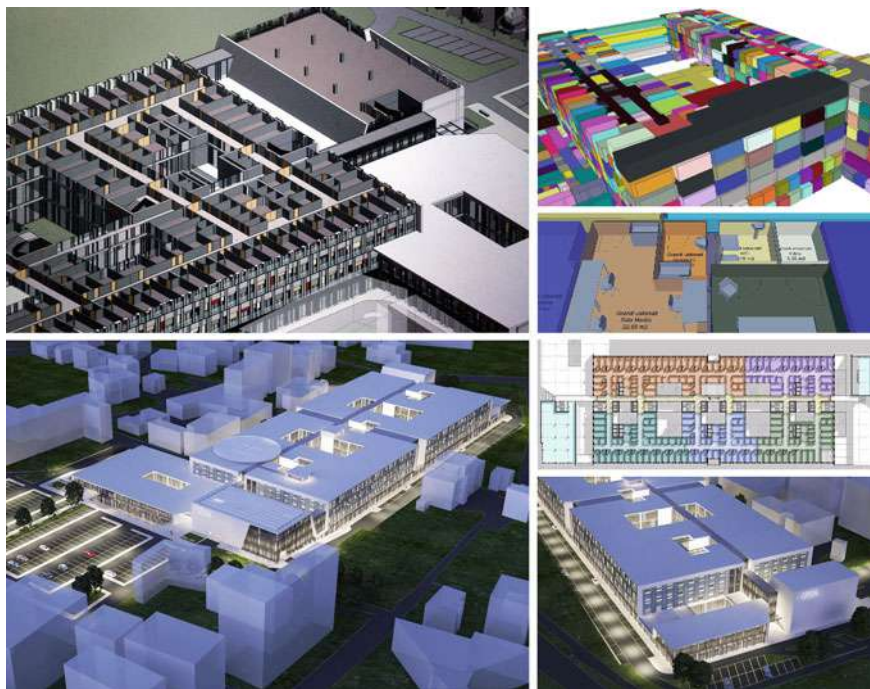
Fig. 3 ARC model of the new hospital center of Lanciano (LOD 200) and space planning optioneering (LOD 100)
