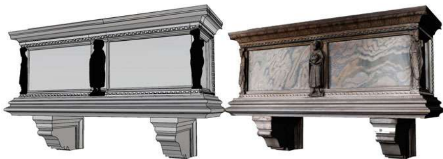
Fig. 3 The same object represented only with geometric information (left) and with texture extracted from georeferenced images (right). Source He.Su.Tech. group
