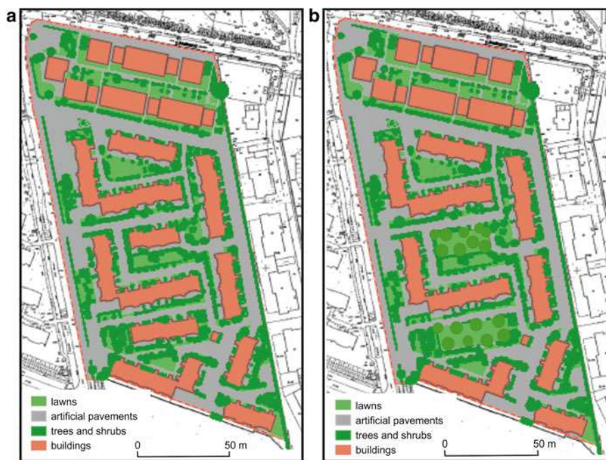
Fig. 11.6 Land cover of Włodarzewska housing estate: (a) – the present state, (b) – changes in land cover proposed in scenario 1 (replacing 2 buildings by lawns and trees)
