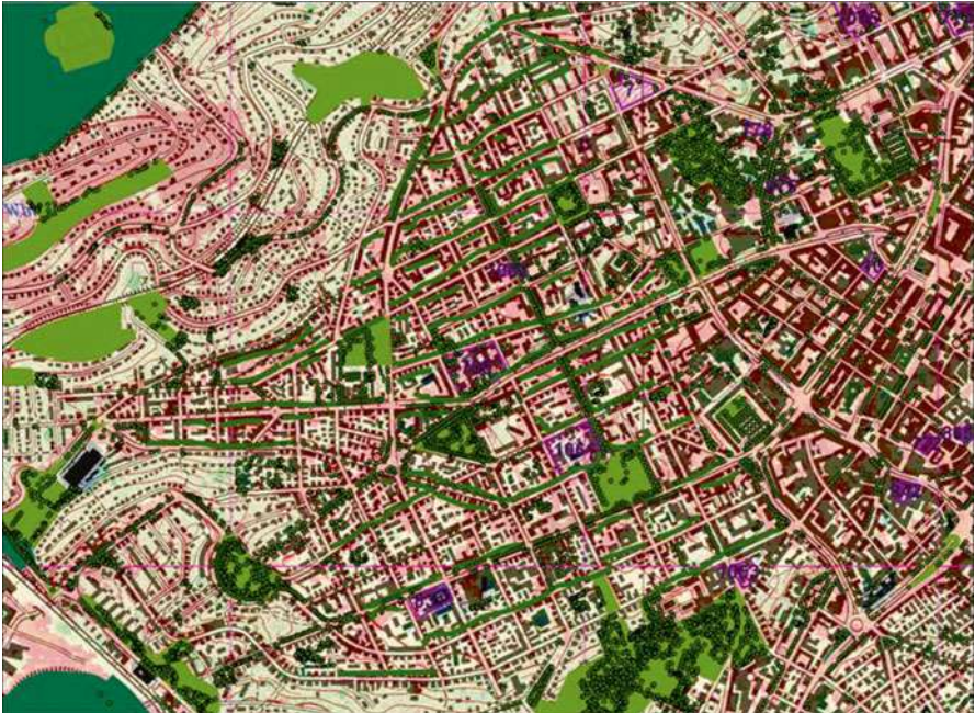
Fig. 10.14 Optimised design of street canyons in Stuttgart-West. Green lines marking street canyons, where the thermal stress is reduced due to facade greening or the use of cool materials for facades. Green circles marking possible positions for trees
