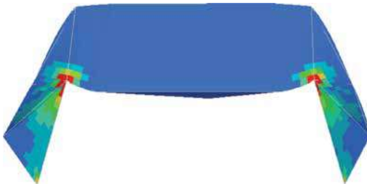
Figure 14. Time domain modal superposition damage result plot. Maximum damage = 116.
