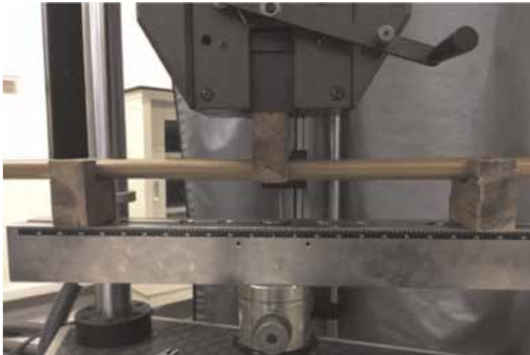
Figure 4. Setup of three-point bending test.
