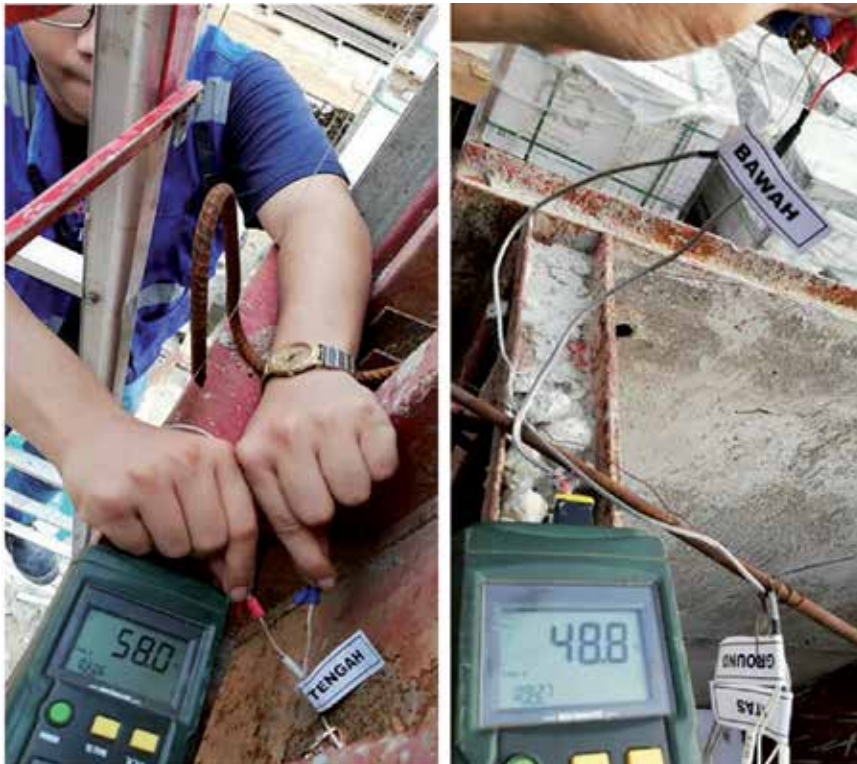
Figure 18. Bioconc LHC mock up thermocouple monitoring.
