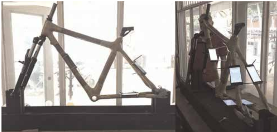
Figure 10. Setup of modal test.
