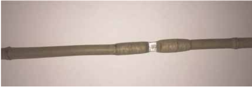
Figure 23. Generic specimen representative of the rear dropout joint.
