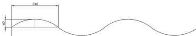
Figure 12. Road profile (distances in mm).
