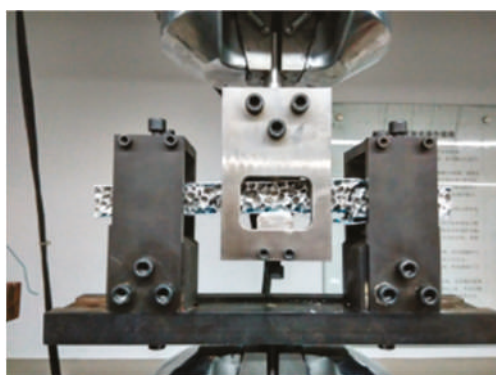
Figure 2. Loading diagram of sample and fixture for fatigue test.
