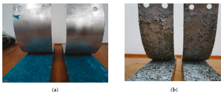
Figure 6. Appearances of Peel Fractures of two types of samples (a) Adhesive joining samples (b) Metallurgical joining samples.
